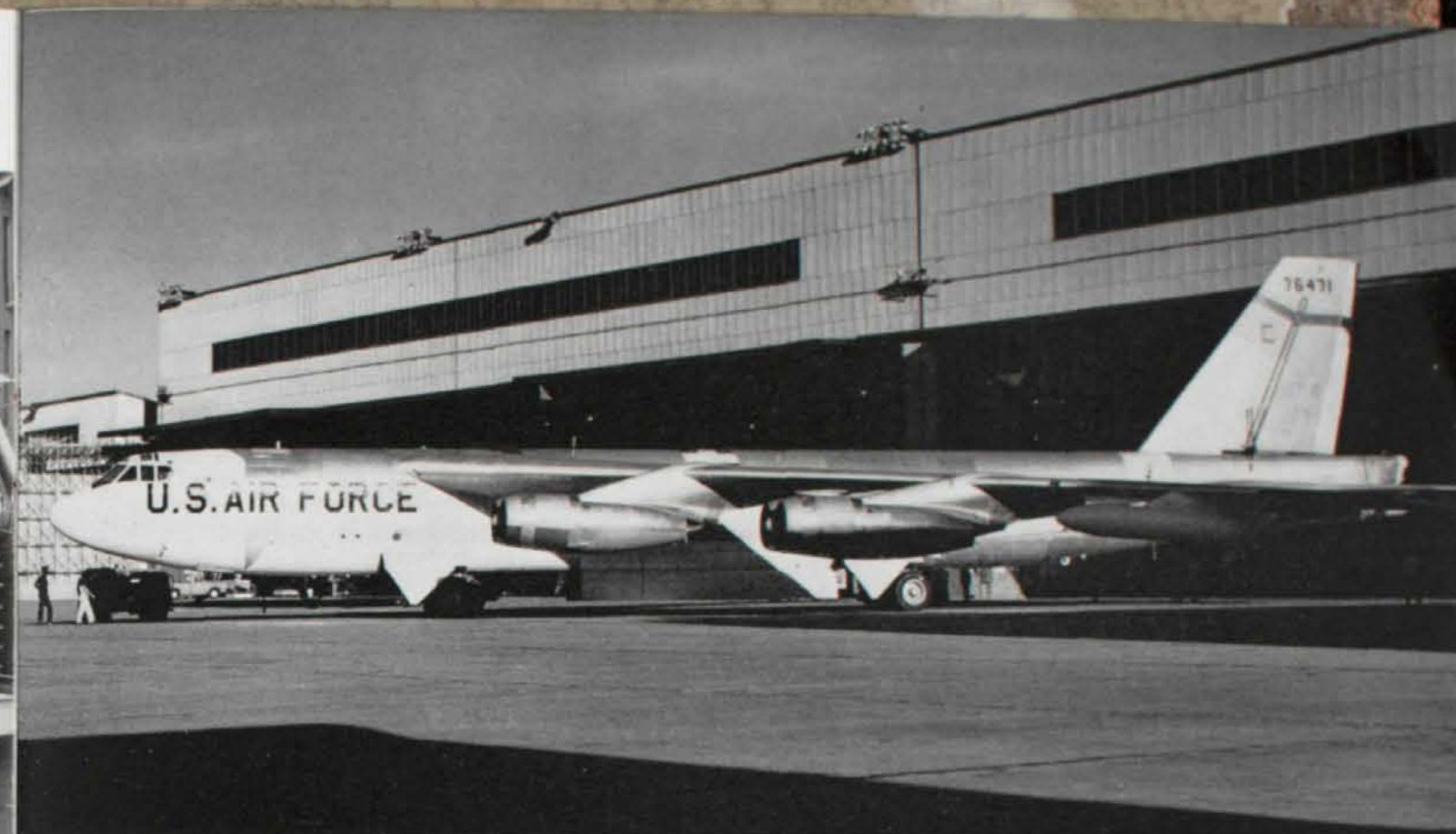
Flight testing of prototype turbofans for the new B-52H, with pods built by Rohr, followed this rollout of a fan equipped B-52G at Boeing-Wichita.
