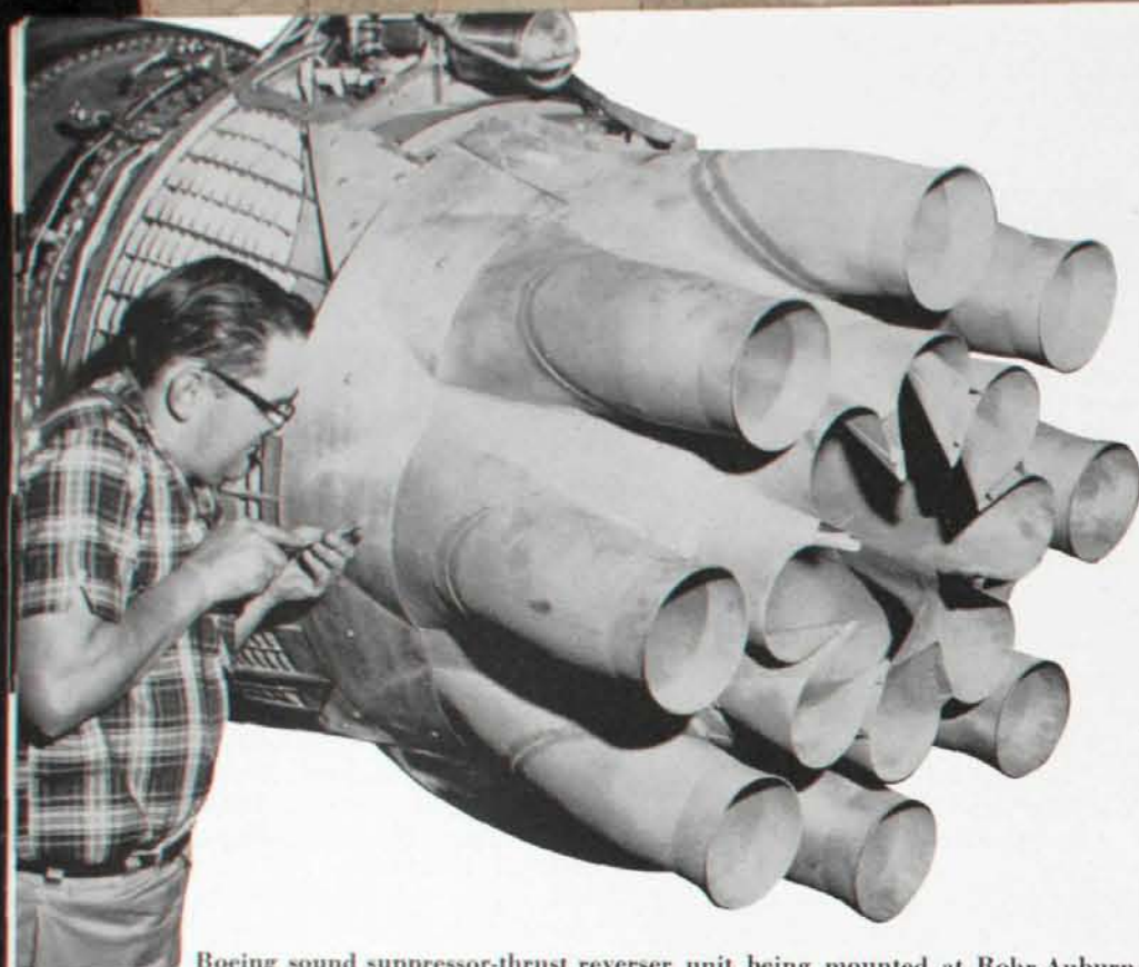
Boeing sound suppressor-thrust reverser unit being mounted at Rohr-Auburn.
