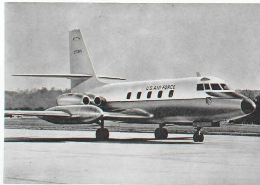
Lockheed's speedy JetStar is the newest plane to carry Rohr jet engine pods.
