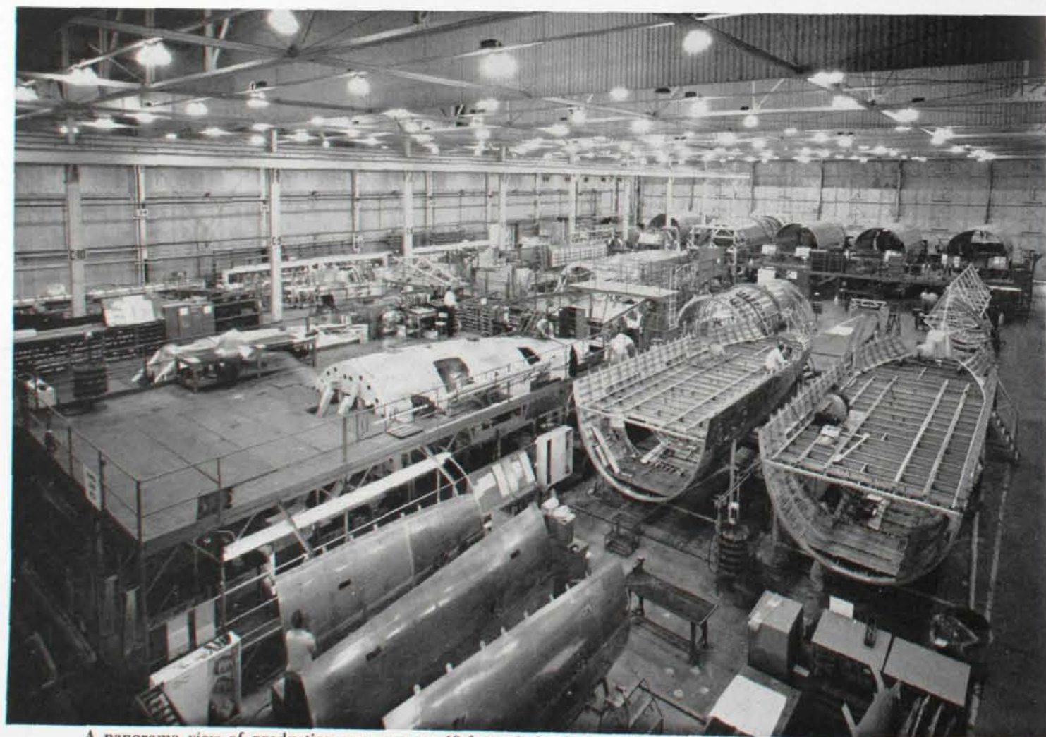
A panorama view of production sequence on 43-foot aft fuselage sections for the Boeing jet airliners.
