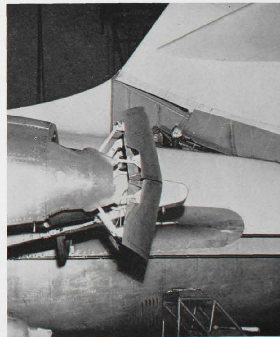
Bonded landing gear door assembly for the Lockheed JetStar.
