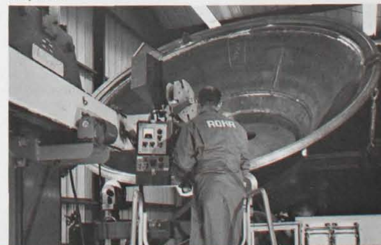
Ablative tape being wrapped to form the non-metallic liner for a Thiokol 156-inch rocket motor nozzle.
