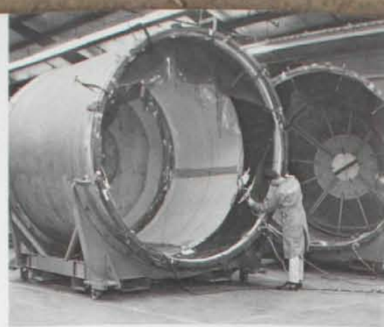
Insulating motor case segments for the Titan III-C solid fuel boosters in the Rohr Space Products Division plant at Riverside.
