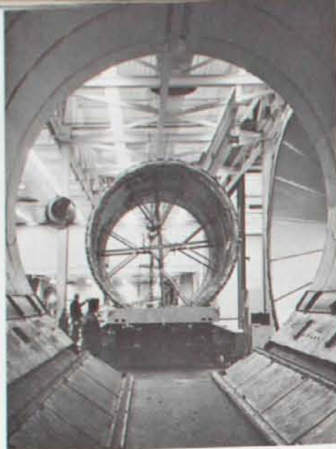
Giant 156-inch motor case entering the autoclave at Rohr Space Products Division for curing and bonding of the rubber insulation.
