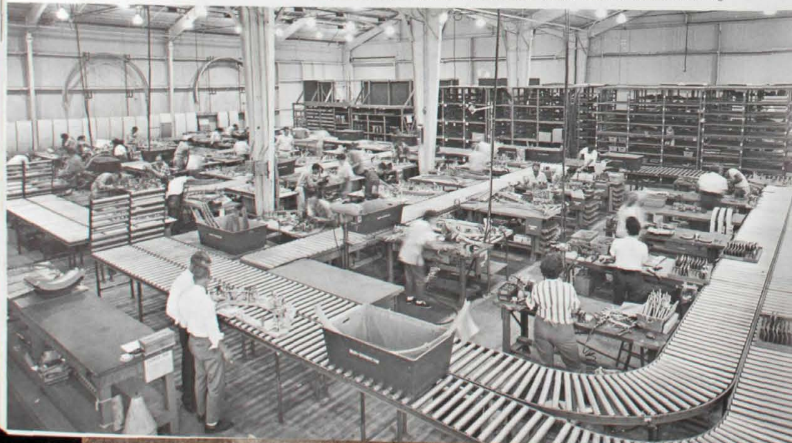
Details moving through extensive roller conveyor system minimize material handling.
