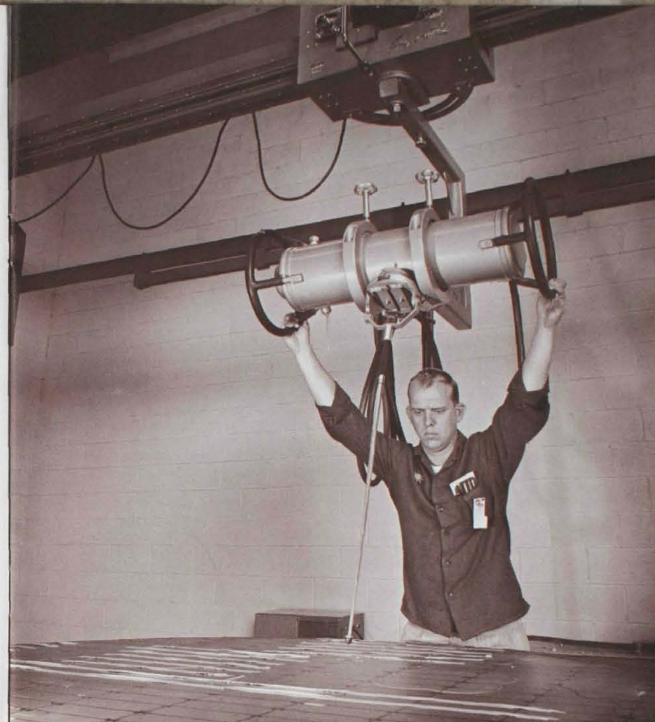
X-ray inspection techniques have been developed to a high level to make possible thorough inspection of such components as this large stainless steel honeycomb sandwich panel.
