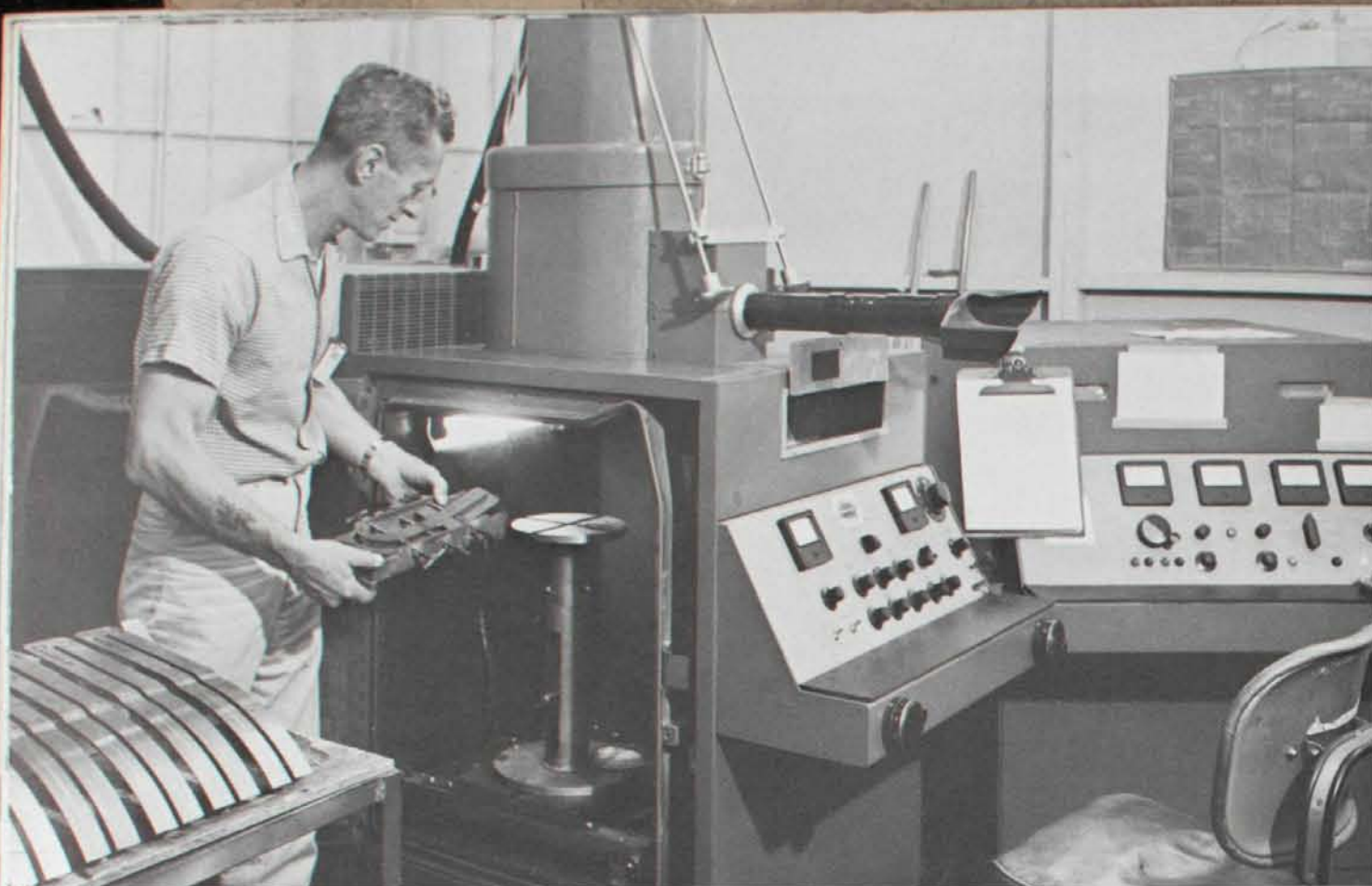
Electron beam welding titanium track fittings. Manufacturing Research efforts have recently enlarged the capabilities of this and other electron beam equipment.
