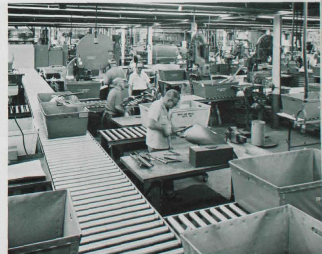
Close-up of parts "kits" on Trim and Drill Department roller conveyor system.
