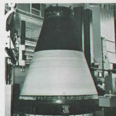
Ablative tape being wrapped to form the non-metallic liner for a Thiokol 156-inch rocket motor nozzle.
