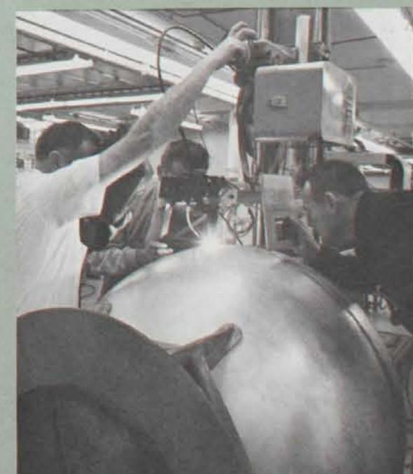
Precise welding was required to join two hemispheres into a perfect sphere.
