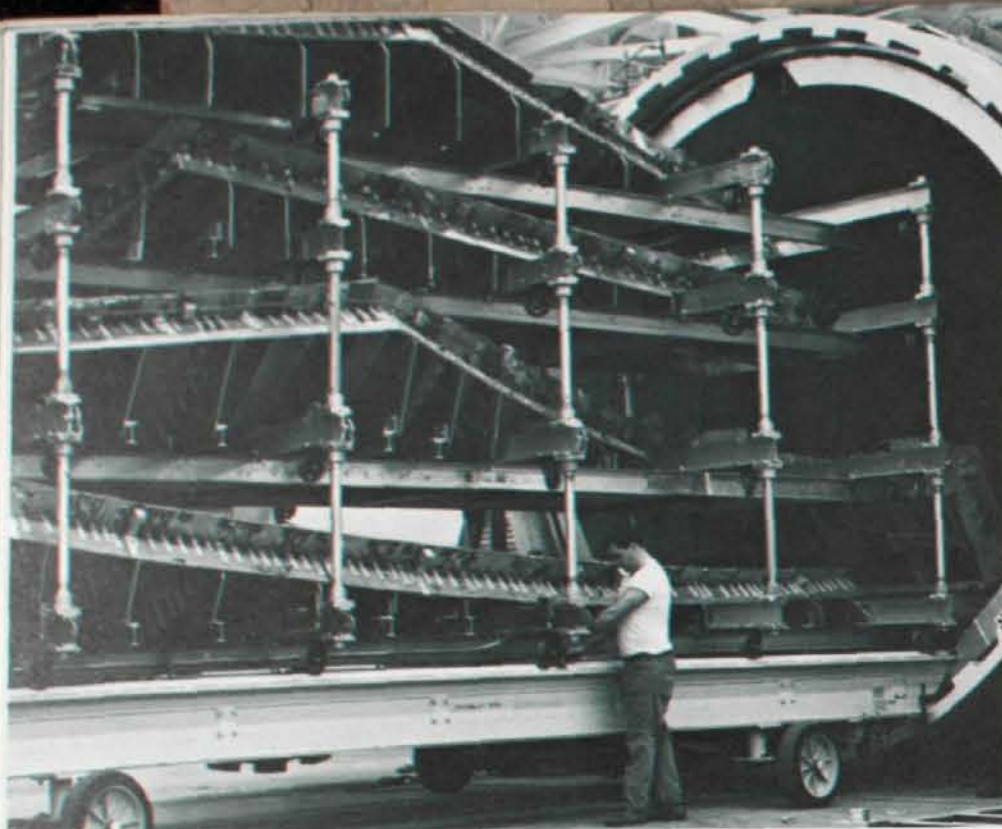
Largest bonded assemblies in the aircraft industry, the C-141 cargo doors enter the 15' x 35' autoclave for bonding on special-built tooling at the Rohr Space Products Division plant in Riverside.
