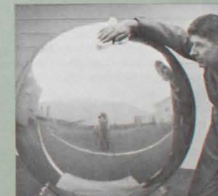
The highly polished surface will reflect signals with sufficient accuracy to allow calibration of radar and radio systems.
