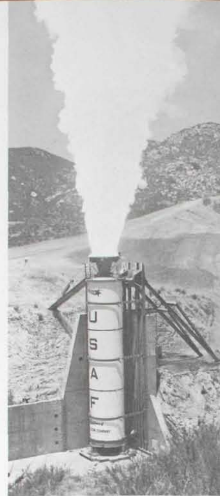
Lockheed Propulsion Company 156-inch solid fuel booster in successful test firing as a part of the U.S. Air Force large solid booster feasibility program.
