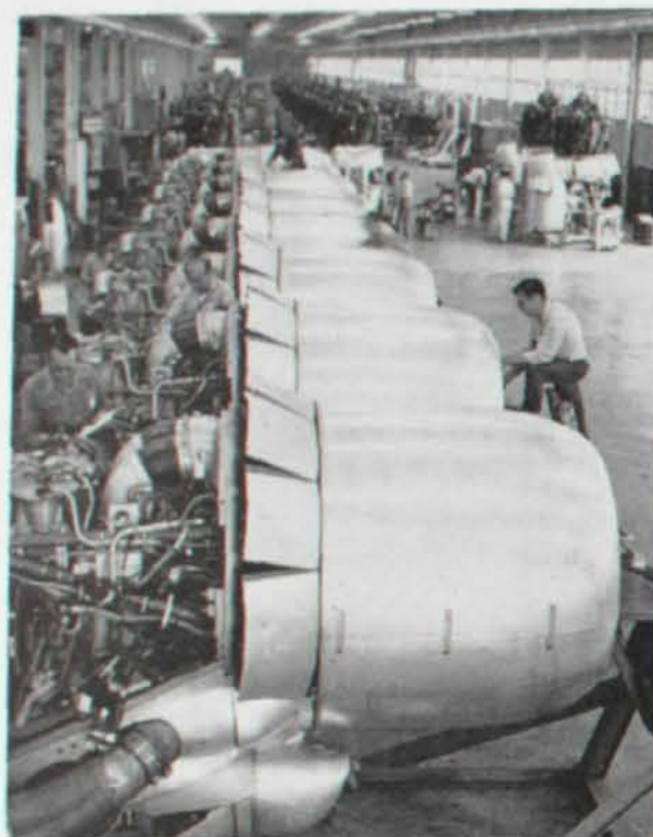
Boeing KC-97 tanker power packs at Riverside.
